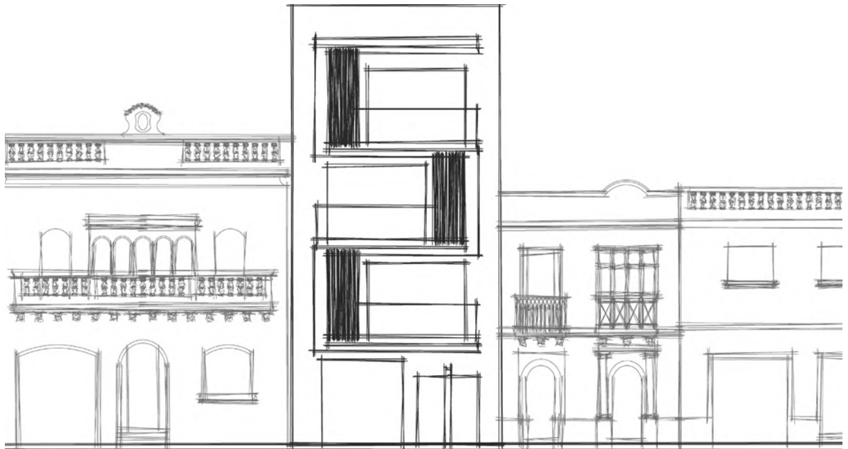
Balconies and façade design incongruous with adjacent buildings
